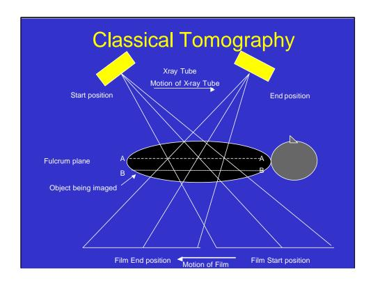
Classical longitudinal tomography used this principle. By moving the x-ray tube and the film such that the central ray from the tube passes through a single point in the image-plane (fulcrum plane), information from the fulcrum plane (A—A) would be imaged sharply o the film, but data from other planes (B—B) would be blurred. Thus although the desired plane was imaged sharply, it was overlaid with extraneous information that often obscured the important detail in the fulcrum plane
