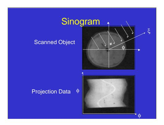
Another concept that is useful to use when considering CT reconstruction is the "Sinogram", which is simply the 2-D array of data containing the projections. Typically, if we collect the projections, using a hypothetical parallel-beam scanning arrangement, using  $\phi$  as the angular parameter and  $\xi$  as the distance along the projection direction, we refer to the  $(\phi, \xi)$  plane representation of the data as the "sinogram".
