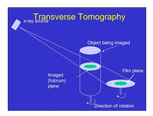
This figure illustrates the geometry of the previous slide. Again, while the fulcrum plane is imaged sharply (because its image rotates at exactly the same rate as the film), structures from planes above and below the fulcrum plane cast shadows that move with respect to the film and therefore the image becomes indistinct as before.
