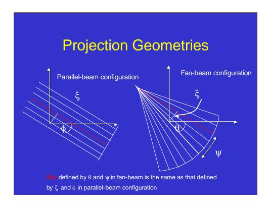
Back to the two geometries. The red ray in both the parallel and diverging configurations are the same, and therefore occupy the same point in sinogram space.
