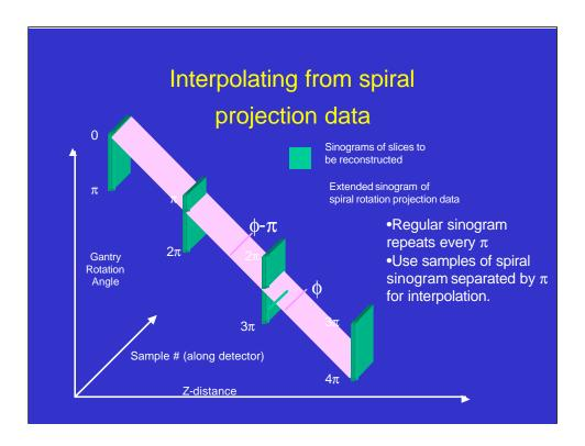
Another way or thinking about this is to imagine that the data from a helical scanner creates an extended sinogram from which conventional sinograms at the appropriate z intervals need to be calculated.
