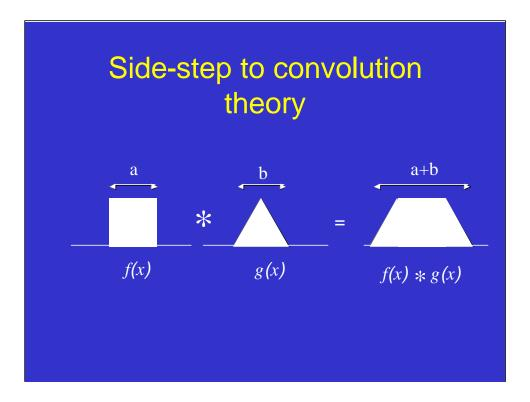
To explain the apparent paradox, we need to revisit an important aspect of convolution theory. When two function are convolved, the result of this operation has a support equal to the sum of the supports of the individual functions. It doesn't matter whether the operation has been carried out in the image domain or the Fourier domain: the result is the same.
