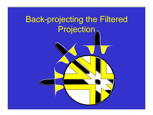
If we now perform the same operation that we performed earlier with the unfiltered projection, we see that the positive parts of the image re-enforce each other, as do the negative components, but that the positive and negative components tend to cancel each other out.
