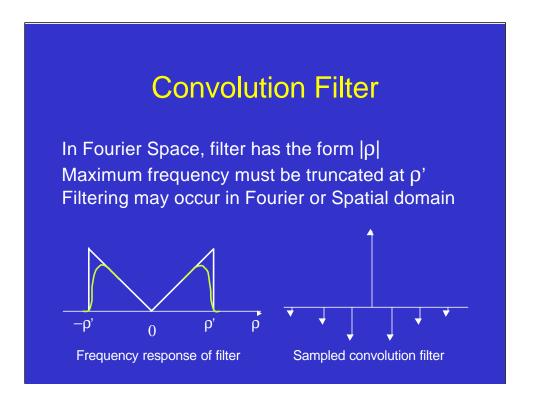
Since the Fourier form of the filter was already shown to be |p|, the spatial form is the inverse FT of this function. The precise nature depends on the nature of the roll-off that is applied in Fourier space, but the net result is a spatial domain function that has a positive delta-function flanked by negative "tails"
