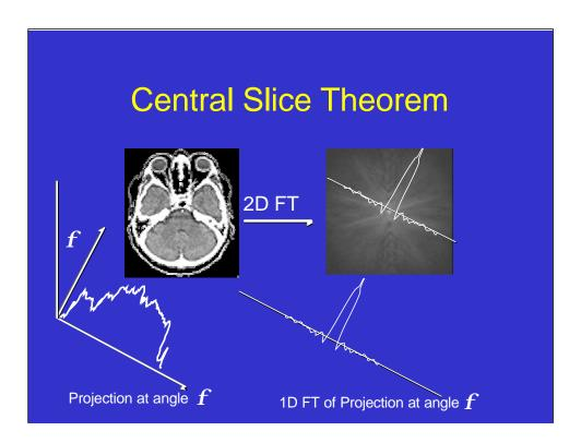
The 1-D projection of the object, measured at angle  $\phi$ , is the same as the profile through the 2D FT of the object, at the same angle. Note that the projection is actually proportional to exp  $(-\int u(x)xdx)$  rather than the true projection  $\int u(x)xdx$ , but the latter value can be obtained by taking the log of the measured value.
