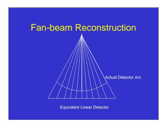
There are two aspects to these formula modifications. First we observe that the equi-spaced data collected on an are are the same as non-linearly —space data collected along a linear detector. We therefore multiply the projection data elements with a 1/cosine weighting factor to reflect this fact.
