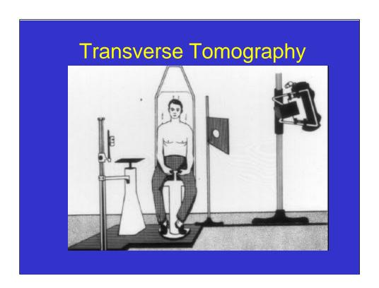
If transverse sections were desired, a different geometry was required. Here the patient and film were rotated while the x-ray tube remained fixed. However the basic principle remained the same: the fulcrum plane was defined by the intersection of the line joining the focus of the x-ray tube, and the the centre of rotation of the film on the pedestal.
