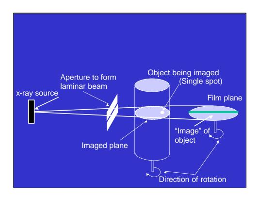
What if we change the geometry of the layergraph so that only a single plane was illuminated? For a single angle of view, a spot in the desired cross-section would project a line over the film. If the object and the film were rotated as before, the lines would intersect on the film to give a blurred representation of the object.
