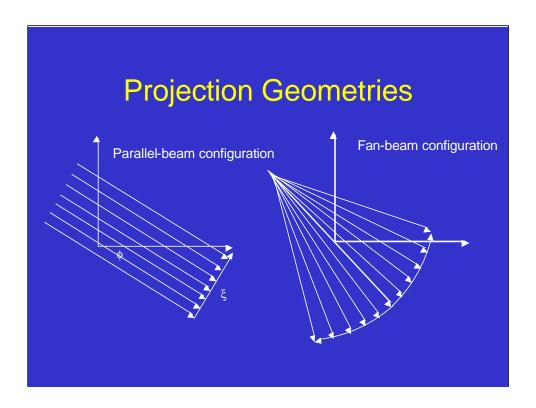
It is worth pointing out that there are two common geometries for data collection; namely parallel-beam and diverging-beam. The parallel-beam geometry was once used in practical scanners, while the diverging-geometry is employed exclusively today. The parallel-beam configuration is useful explain the concepts; allows simpler reconstruction algorithms, and is often the form to which diverging-ray data are converted prior to image-reconstruction.
