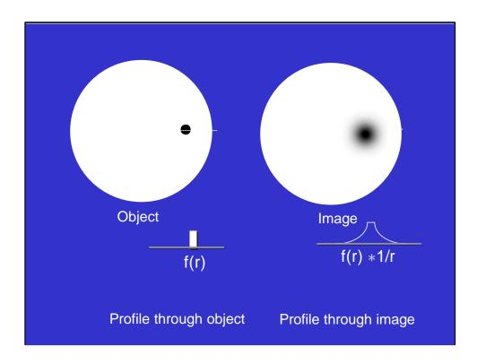
And after a full rotation of the film and the object, this pattern would become a diffuse blur. The nature of the blur can readily be shown to be = 1/r. Thus any structure in the cross-section is recorded on the film as a result of a convolution of the original cross-section with the two-dimensional function 1/r.
