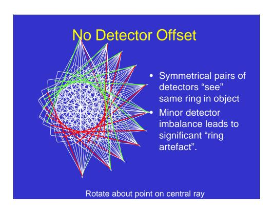
As we rotate the gantry through 180 deg, these pairs respond mainly to data lying on rings. Incidentally, detector imbalance generates "ring-artefacts" in the images.
