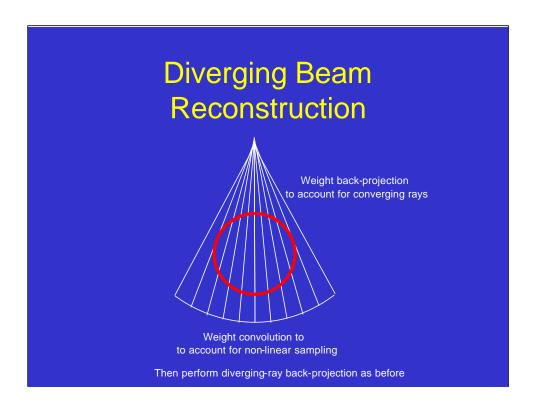
Also, since the rays become closer together as they approach the source, we must incorporate an inverse quadratic weighting factor in the back-projection to account for this "bunching-up" of the rays.
