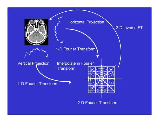
If all of the projections of the object are transformed like this, and interpolated into a 2-D Fourier plane, we can reconstruct the full 2-D FT of the object. The object is then reconstructed using a 2-D inverse Fourier Transform.
