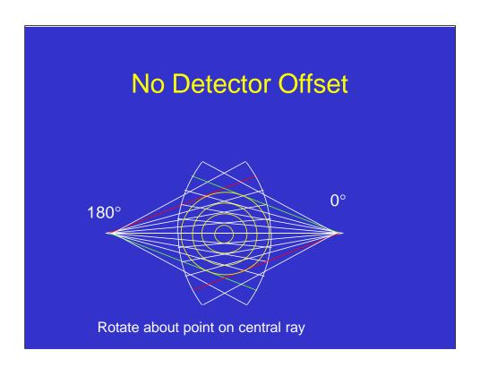
If we rotate a 3<sup>rd</sup> generation system about the central ray, it is clear that detectors symmetrically placed about the central detector, mostly "see" the same annulus of data in the image.
