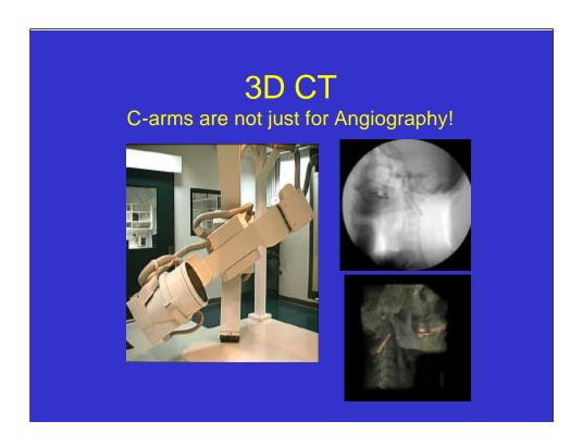
Typical 3D cone-beam CT scanners are built around standard C-arm angiographic systems.
