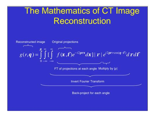
The mathematics of the image reconstruction process, can be expressed compactly in the above equation, where the terms have been grouped to reflect the "filtered-back-projection" approach
