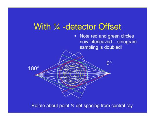
However, if we offset the detector by ½ of the detector spacing, we see that the same pairs of detectors now see different annuli. Thus we have effectively doubled the sampling without any cost to the system except that we must scan the full 360 degrees, rather that the 180 deg + fan angle that is all that is necessary with the symmetrical configuration.
